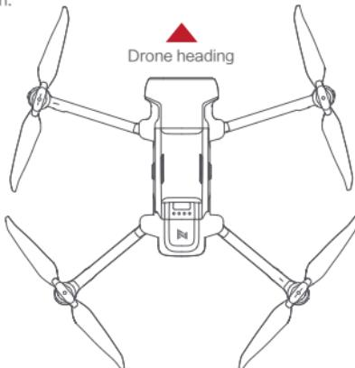
⚠ · Safety tip: Keep the tail facing the operator when maneuvering the craft to avoid misjudging the direction.
