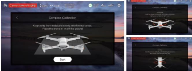
⚠ - If calibration fails multiple times, update the calibration site.
