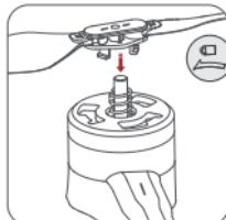
Note: This example is for counter-clockwise propeller installation.
