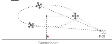
If sticks are moved in flight, the flight altitude or radius will be changed.
