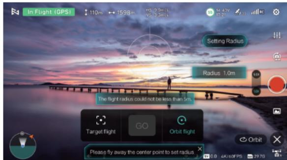
During the orbit a point flight, you can set the steering and speed of the go-around flight on the Fimi Navi 3.0 APP, and click "X" to exit the orbit a point flight.
