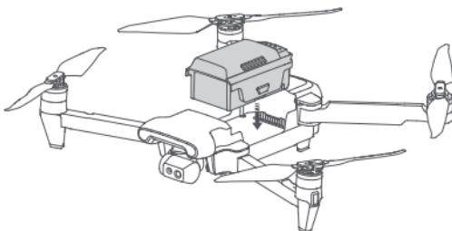
Installing the Battery
