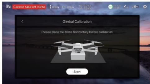
⚠ - Please connect the airplane and gimbal before calibration, gimbal calibration can not be done in flight.
