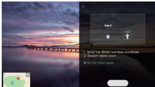
The interface of map transmission shows the coordinates of the aircraft and the current time in real time, and supports the functions of map transmission screen indentation and screenshot.
