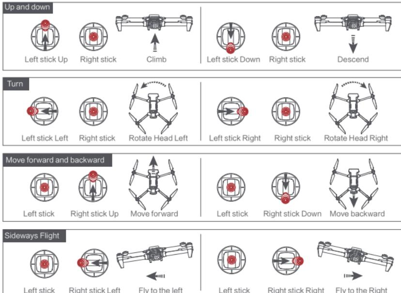
⚠ - Remote control joystick settings can be changed in the remote control setup menu (default is US hand)
