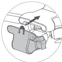
Remove the gimbal protector as the arrow leading
